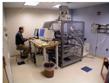
Fig. 2. The HUCAPS aerosol output is introduced into this chamber designed for human subject studies.
