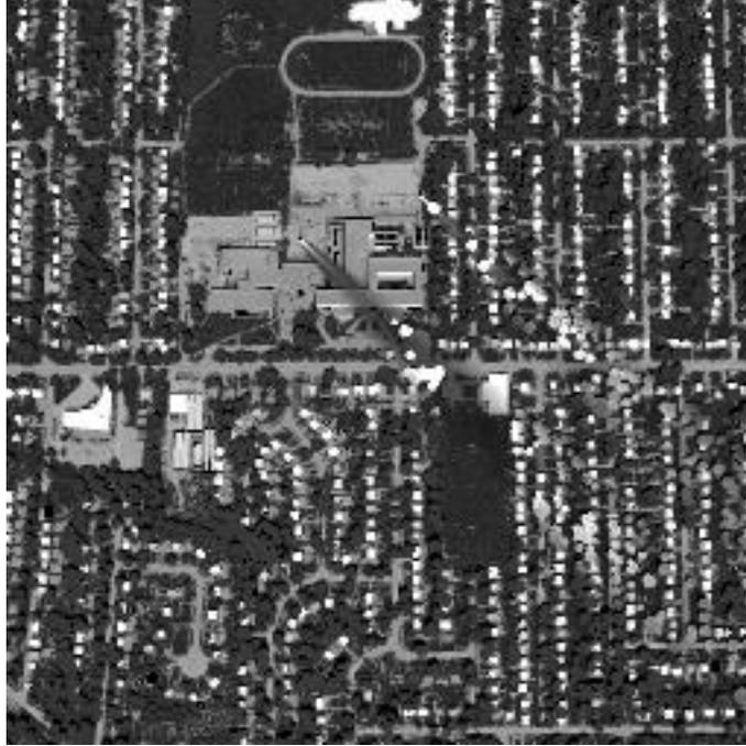
**Figure 1.** Single-band image of synthetic DIRSIG data at  $10.73\mu\text{m}$ . Both plumes can be seen moving from the middle of the scene to the upper-right corner. The  $\text{NH}_3$  plume is the left-most plume while the freon-114 plume is on the right.
