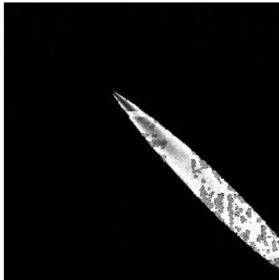
Figure 9. The freon-114 detection map for the mixed gas in a strong release.
