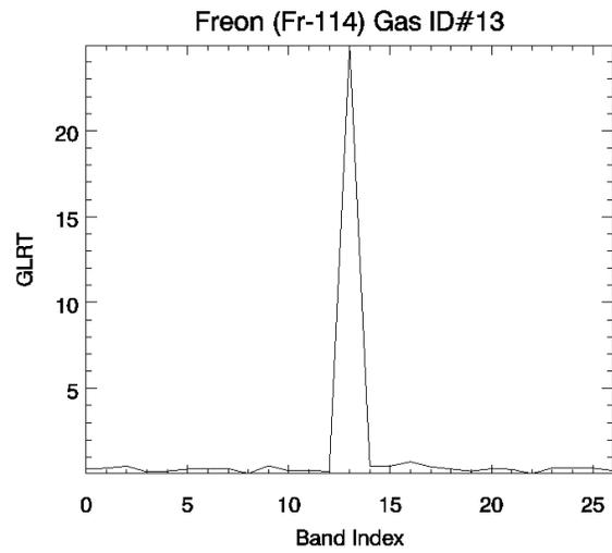
**Figure 5.** GLRT results for a pixel in the freon plume for all gases in the target set. Freon is gas no. 13.
