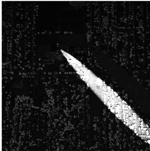
**Figure 8.** Detection map resulting from application of the  $\text{NH}_3$  target space to the image.
