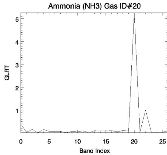
**Figure 7.** GLRT results for a pixel in the  $\text{NH}_3$  plume for all gases in the target set.  $\text{NH}_3$  is gas no. 20.
