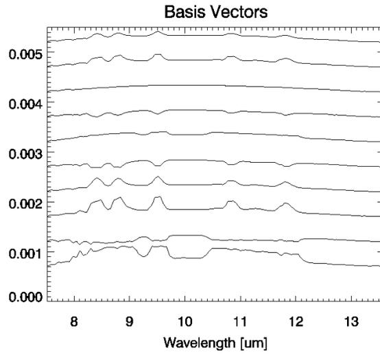
**Figure 2.** Target basis vector set resulting from application of the MaxD algorithm to the freon target space (plots are offset for clarity).
