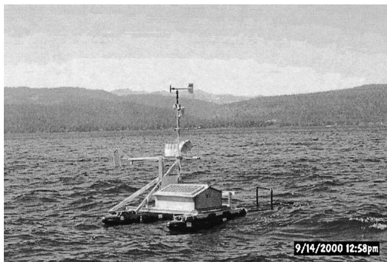
FIG. 2. Surface monitoring station at TR3. The station measures the radiometric skin temperature, bulk temperature, wind direction (magnetic) and speed, relative humidity, air temperature, and net radiation.
