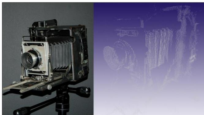
"This image shows the automated process of extracting a three-dimensional model of an object using a low-cost homemade 3d line scanner. The scanner uses structured light from a projector and a calibrated camera to extract a 3-d point cloud that is faceted and mapped with an image of the object."
