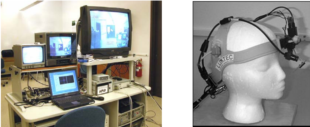
Figure 1 ASL Series 500 eyetracker system (left) and Model 501 headband-mounted optics (right)
