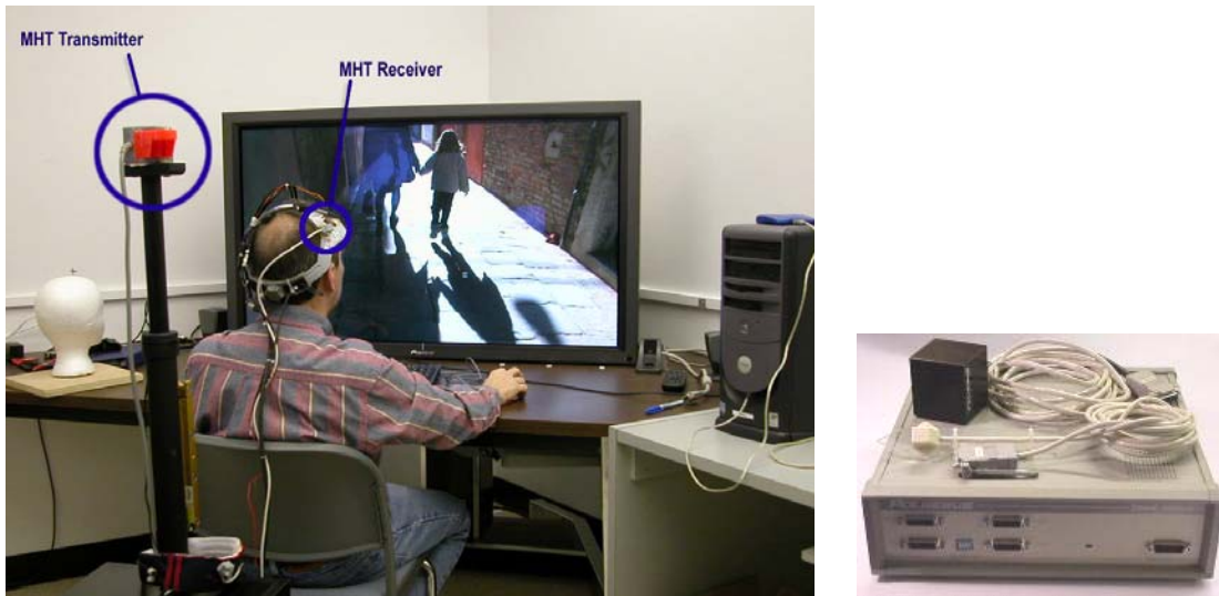
Figure 3 Polhemus Fastrak magnetic-field head tracker
