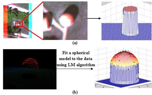
**Figure 5. The hemispherical dome of RIT Observatory can be modeled by fitting a spherical surface to lidar point cloud (b) but can not be modeled from passive imagery (a)**
