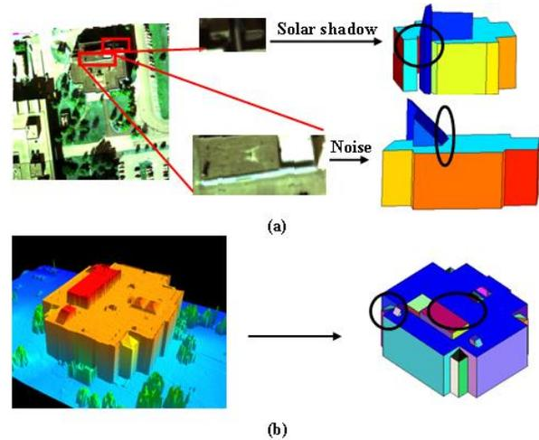
**Figure 3. (a) Artifacts in 3D model of RITs Center for Imaging Science built from passive video due to solar shadows and noisy edges (b) Accurate 3D model of the same building built from lidar point cloud**
