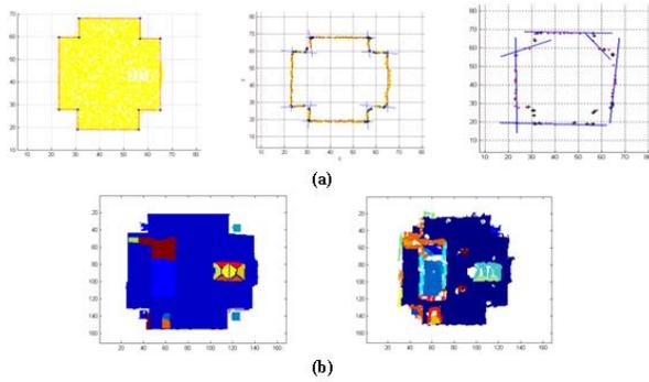
**Figure 4. (a) Images showing the edges extraction using outer boundary analysis when lidar point cloud is adequately sampled, sampled at half the rate and sampled at quarter the rate. (b) Images showing failure of segmentation in inner boundary analysis due to undersampled lidar data**
