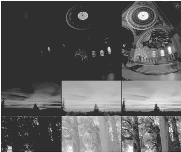
**Fig. 7** Three HDR images from [www.debevec.org](http://www.debevec.org). The leftmost column illustrates linear rendering of the image data, the middle column illustrates manually optimized power function transformations, and the rightmost column represents the automated output of the iCAM model implemented for HDR rendering (see Fig. 3).
