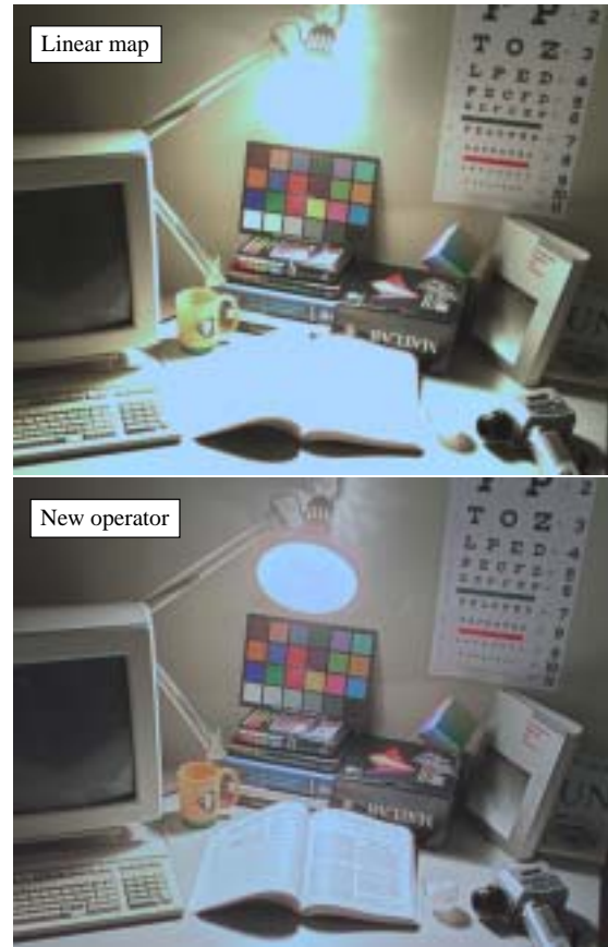
Figure 1: A high dynamic range image cannot be displayed directly without losing visible detail using linear scaling (top). Our new algorithm (bottom) is designed to overcome these problems.
