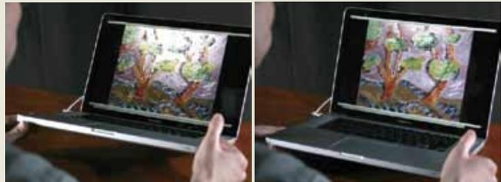
**tangiBook in Action:** Using an accelerometer, webcam, and custom software, the tangiBook tracks the orientation of the laptop screen and the position of the observer in real time. Tilting the laptop (as shown) or moving in front of the screen produces realistic changes in surface lighting and material appearance.
