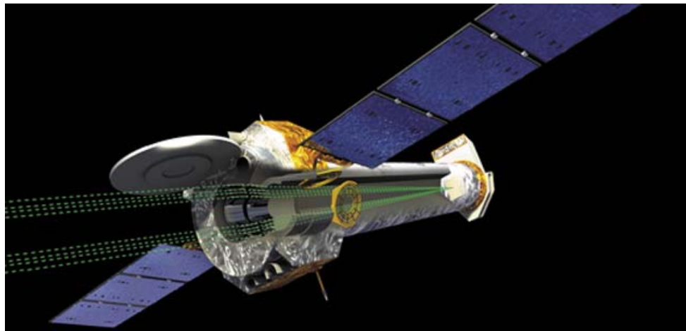
Grazing incidence optics used to focus X rays in Chandra orbiting X-ray observatory
