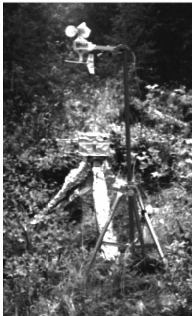
**Figure 1:** A weather station/situation monitor deployed on a wildfire in Montana (Cooney Ridge Complex). The weather station is in the foreground; the other tripod mounts another experiment. The data logger is buried about 10 cm underground to protect it from the fire front.
