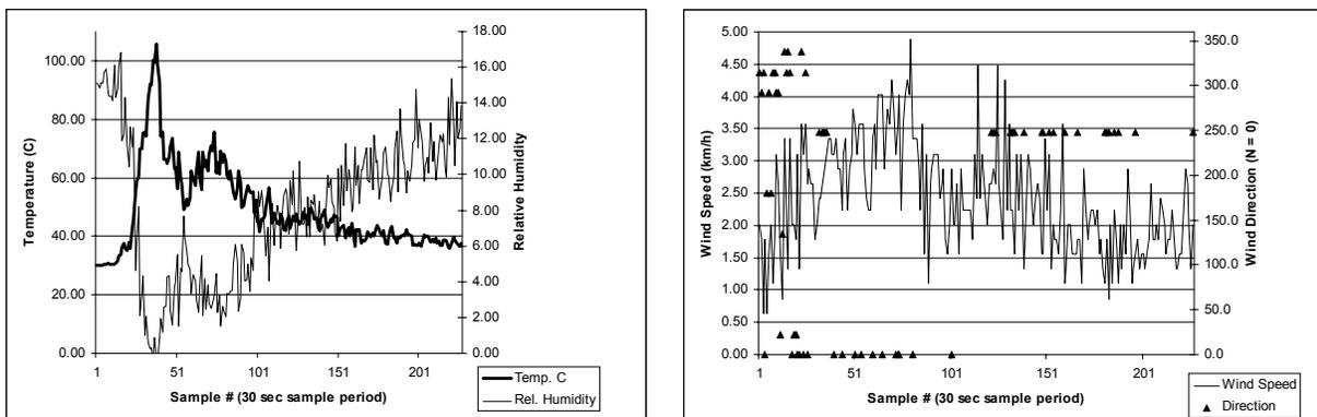
**Figure 4:** A plot of the relative humidity and air temperature (left) and wind speed and direction as a function of time (right) as a function of time. The wind direction changed from west to directly toward the fire ( $0^{\circ}$ ) during the time of fire passage. The fire front passed the mast system at about sample 40. Note the precipitous drop in relative humidity and increase in temperature during fire front passage.
