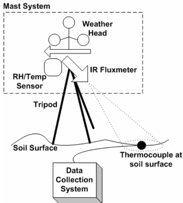
**Figure 2:** An IR flux meter, relative humidity sensor, temperature sensor and wind vane (speed/direction) are mounted on a tripod about 2 m above the surface of the soil. ('mast package') The flux meter field-of-view is centered on a thermocouple that is in contact with the soil surface. The data from both sensors is logged as a time series by a buried 'data collection system'. Up to 3 additional sensor pairs and two additional thermocouples may be logged by a single logger.
