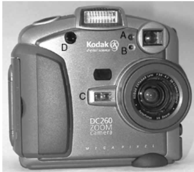
Figure 3: Kodak DC260 (A-Ambient light sensor, B-Flash sensor, C-Autofocus sensor, D-Self timer light)
