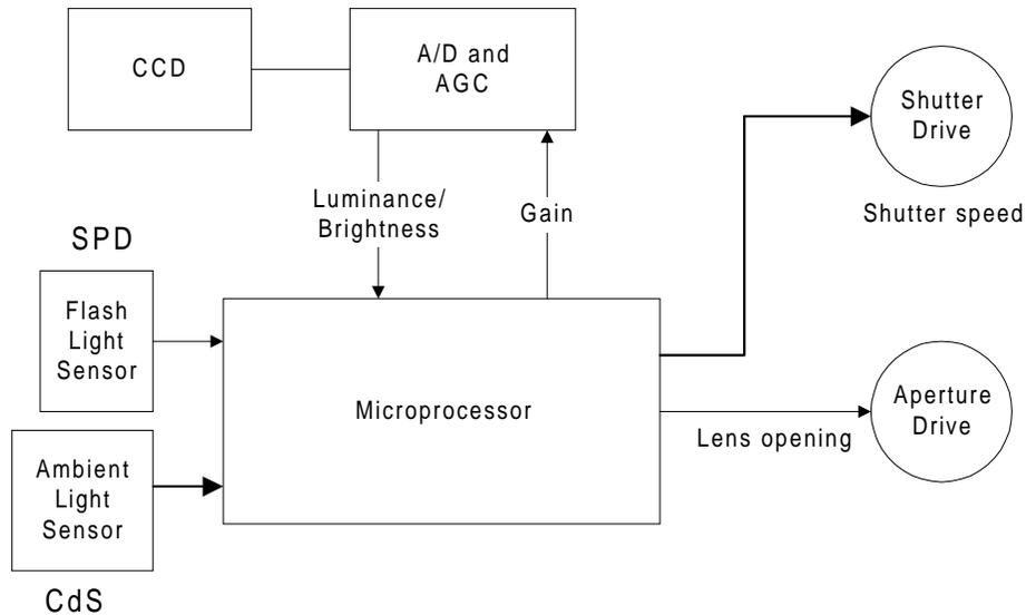
**Figure 5: Expanded view of an AE subsystem**
