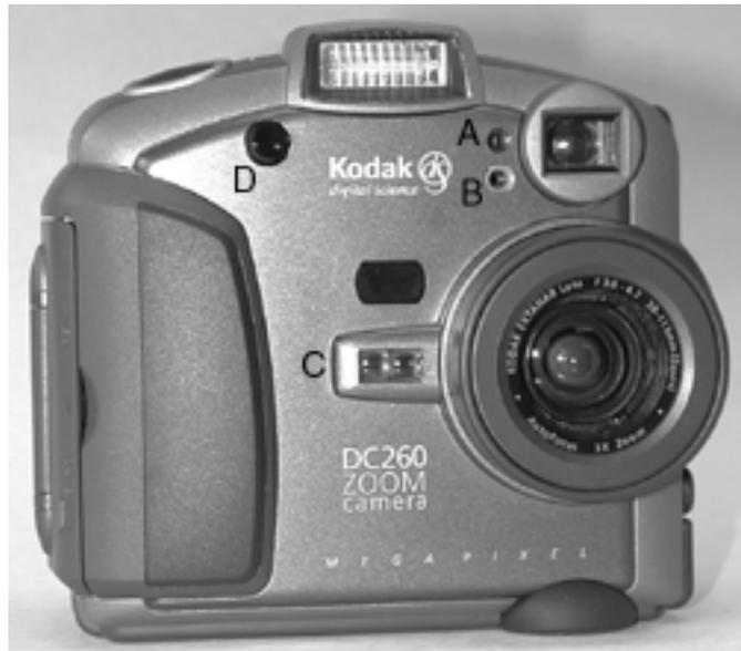
**Figure 3: Kodak DC260 (A-Ambient light sensor, B-Flash sensor, C-Autofocus sensor, D-Self timer light)**
