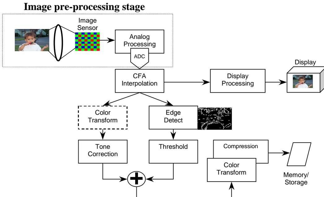
**Figure 1: Image processing pipeline in a digital camera**
