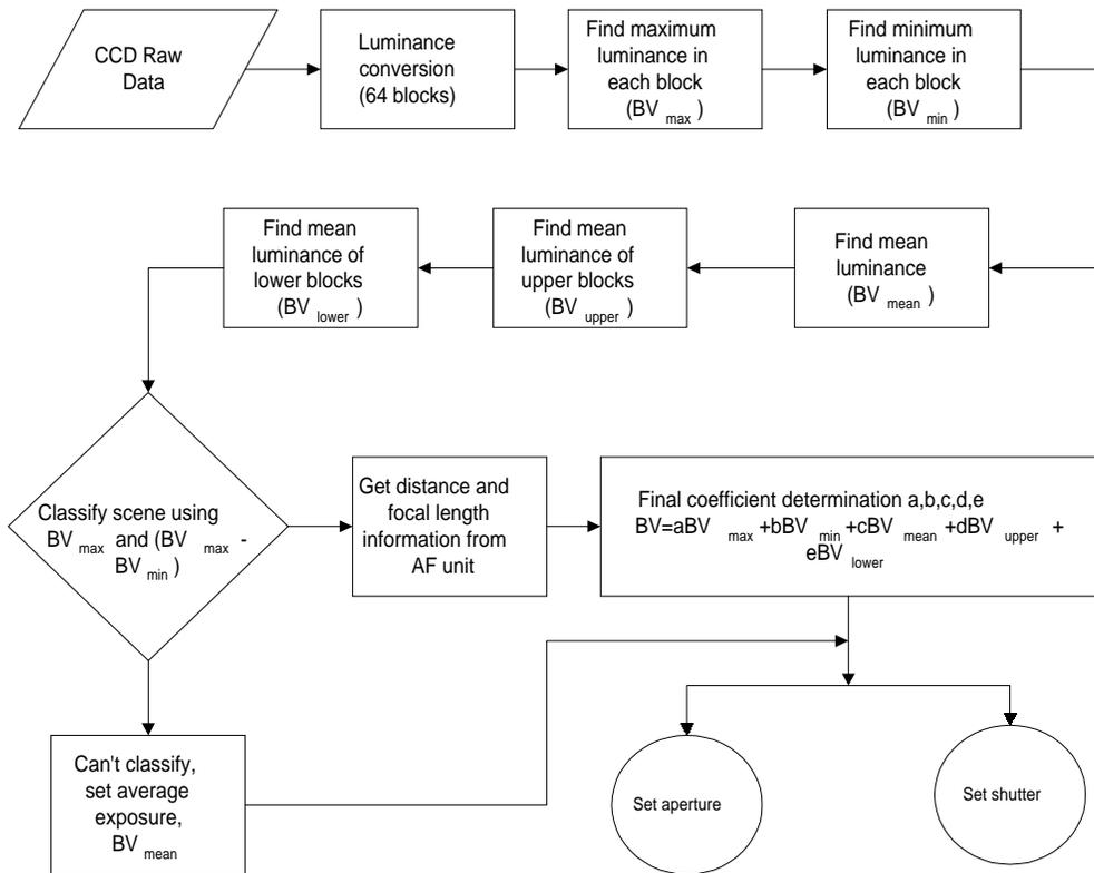
**Figure 4: Sample algorithm using scene segmentation in automatic exposure development**
