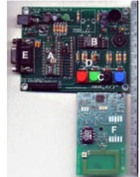
A prototype AFD with microprocessor and radio transmitter sub-units. A- Microprocessor; B- Analog processing; C- Input switches; D- Status LEDs; E- GPS communication port; F- RF communication deck
