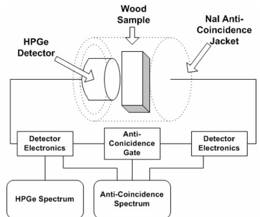
**Figure 2 - High purity germanium detector with anti-coincidence jacket**
