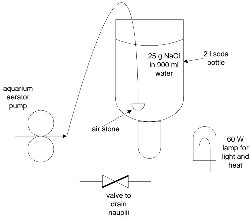
**Figure 14 - Hatching and rearing setup for *Artemia salina*.**
