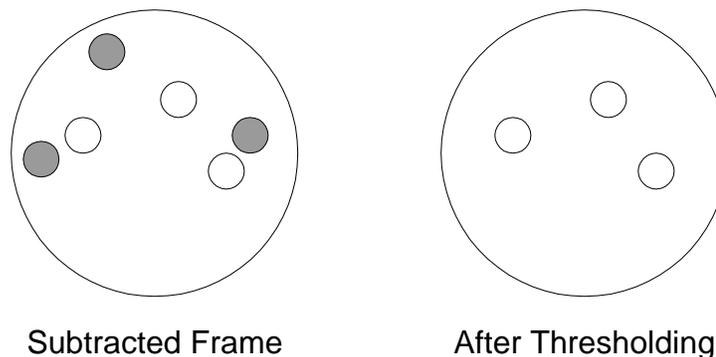
**Figure 4 - Eliminating negative pixels (negative pixel thresholding) eliminates double counting of live plankton.**
