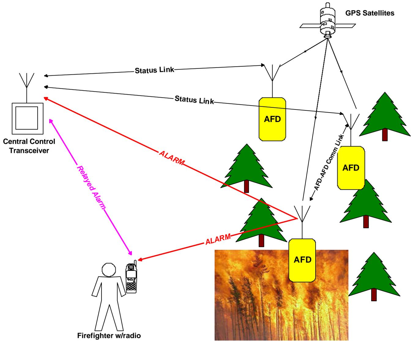
Figure 1 - Deployment and communication between AFDs and base units, other AFDs and firefighters in a fully networked system.
