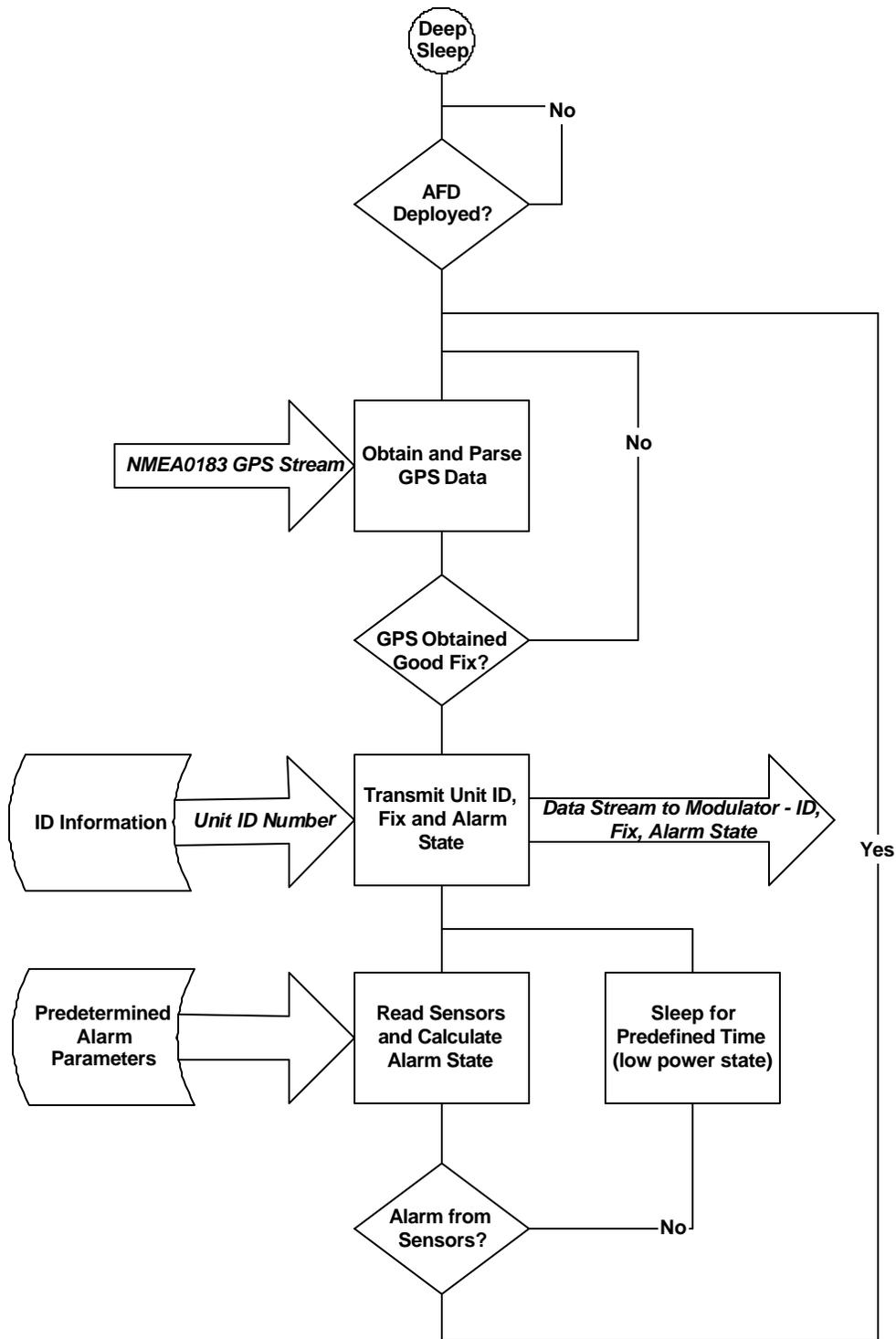
Figure 6 - Software flow diagram for the AFD prototype. The software makes use of the powerful instructions in the Parallax, Inc. PBASIC programming language.
