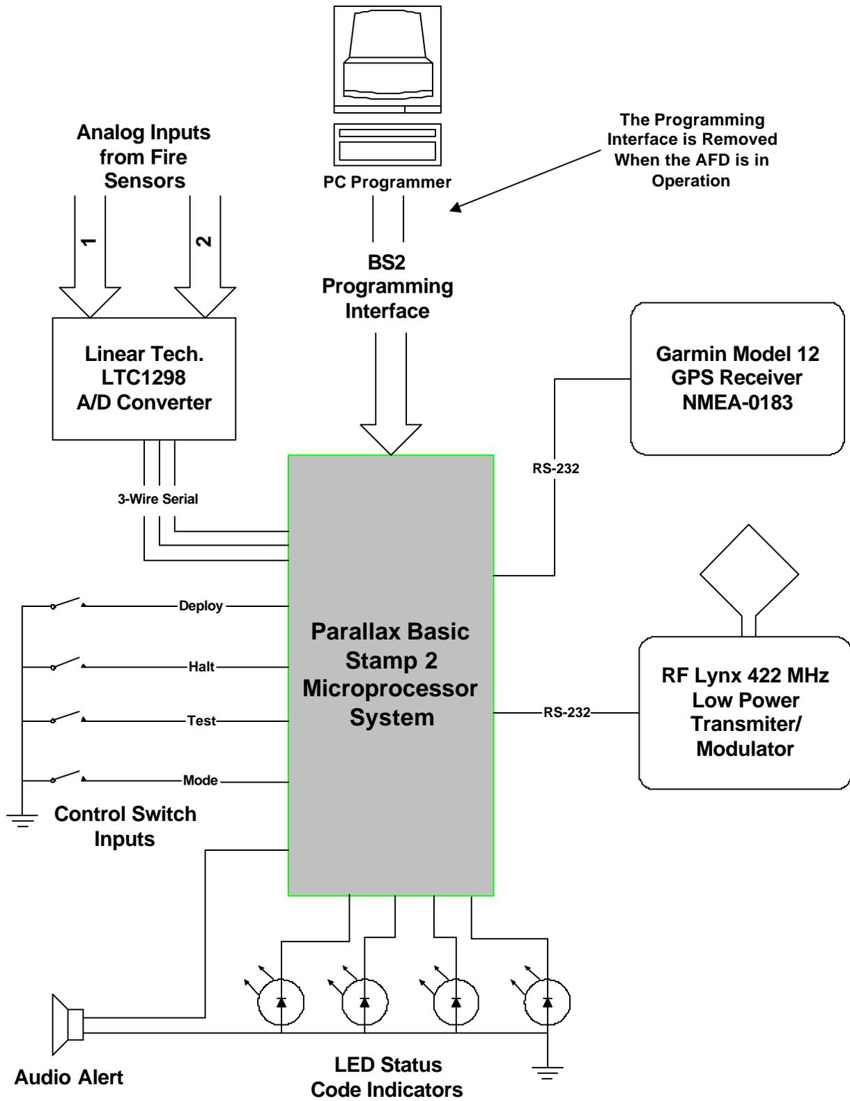
Figure 5 - Detailed block diagram of the prototype AFD. Fourteen of the sixteen available input/output pins of the BS2 are used in this application.
