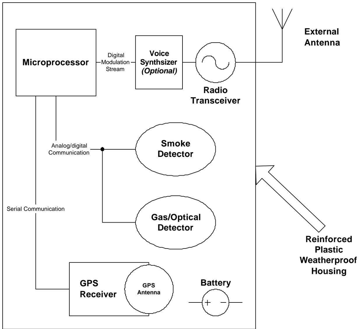
Figure 3 - Block diagram of the AFD, showing the logical and signal interconnections between the fire sensors, global positioning system receiver, radio transceiver and power system.
