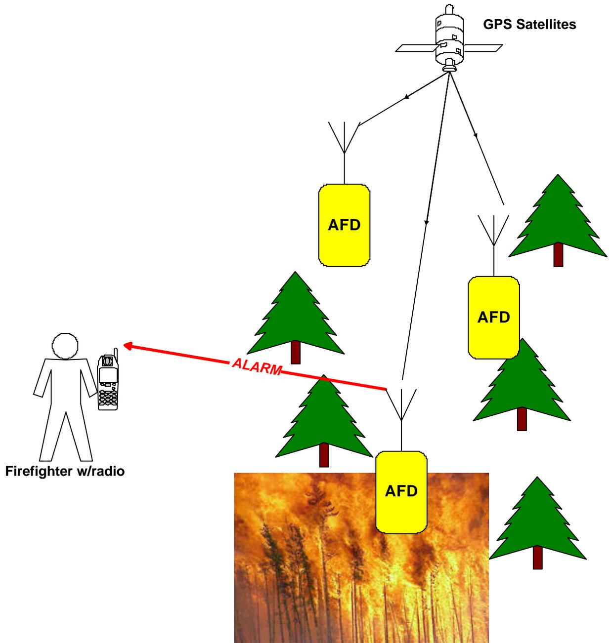
**Figure 2 - Simple direct voice AFD operation. The AFDs report via synthesized voice messages directly to radio receivers at the fire site.**
