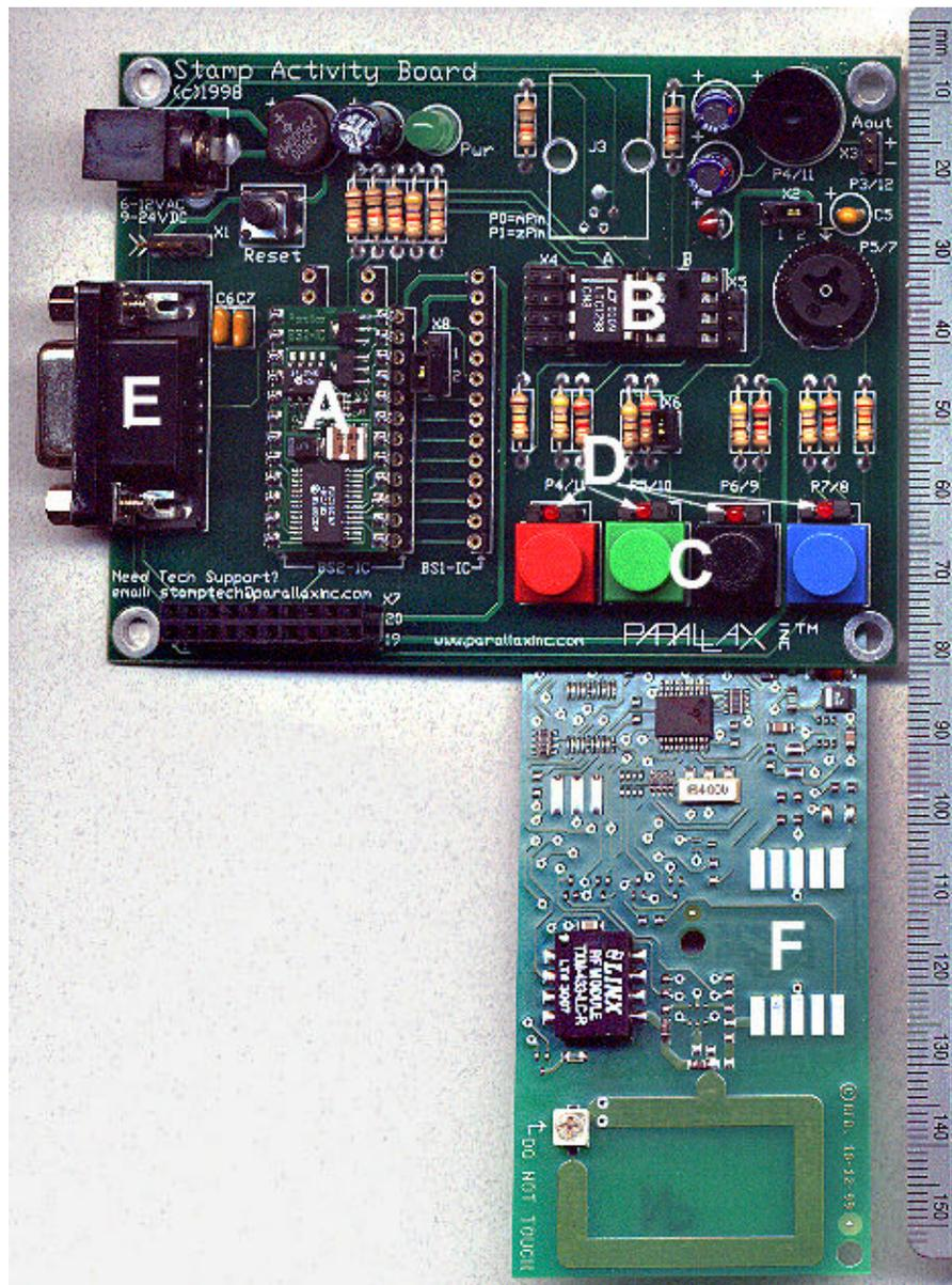
Figure 4 - Photograph of the prototype AFD. A - Parallax Basic Stamp microprocessor; B - Linear Technology LTC1298 2-channel analog-to-digital converter; C - Input switches for start-up, deactivation and test; D - Status LED indicators; E - Programming and GPS communication ports; F - RF communication deck.
