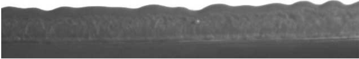
Figure 6. An optical microscope image of the side profile of vinyl siding.
