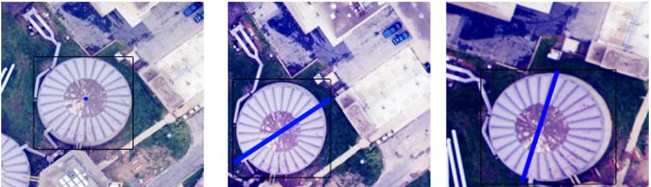
Figure 8 – Left: Target with single point chosen. Middle/Right: Corresponding epipolar lines.
