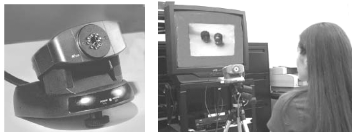
Figure 1. The ‘remote’ eye camera (left) is placed just below the subject’s line of sight (right). The lens is surrounded by infrared emitting diodes to provide coaxial illumination.
