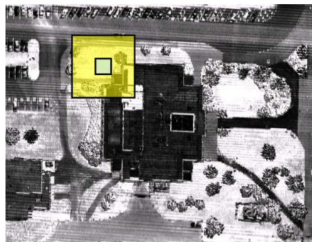
Figure 4. Illustration of the Modified Median Filter at a single location; median height value is calculated in smaller window, points 3m above median in larger window are flagged as non-ground points
