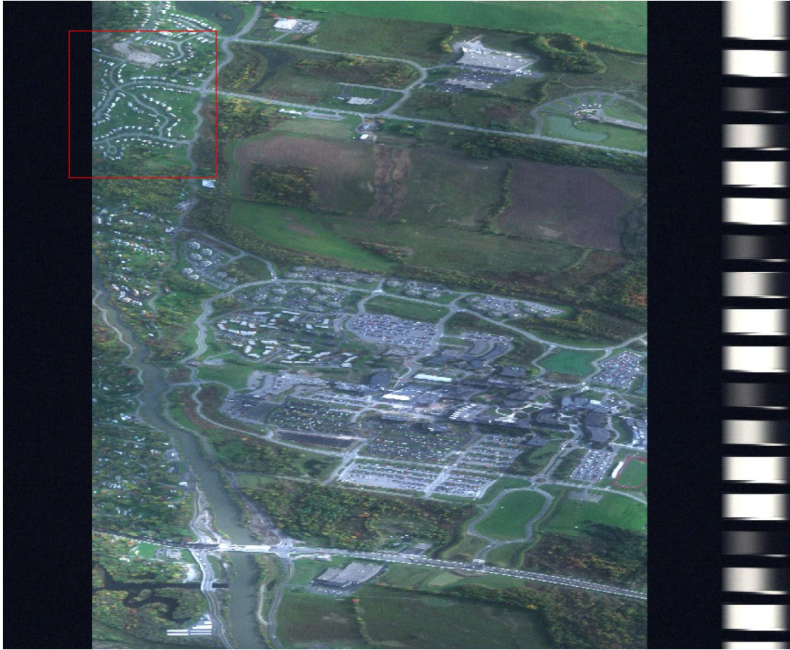
Figure 2. Raw, un-roll-corrected color rendition of the scene of interest taken by MISI.
