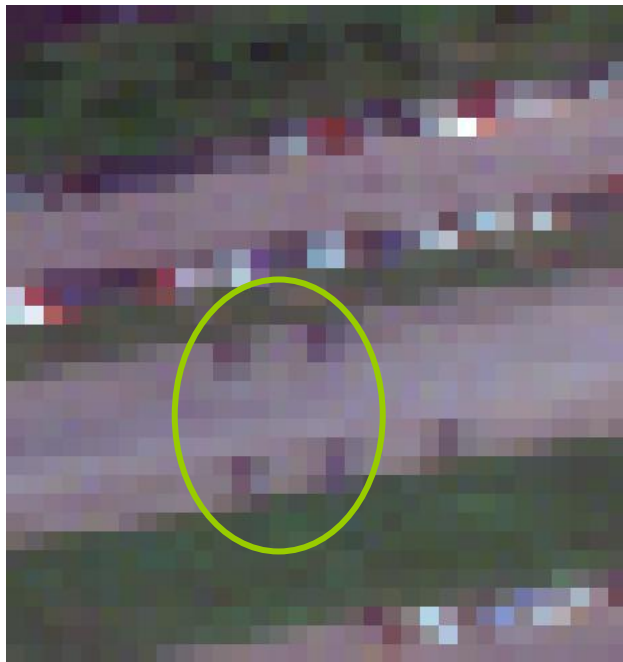
Figure 6. The oval on the zoomed MISI image (12:09 pm) in the lower left encircles the four blue cars shown in the second row of the upper photograph. The lower right image is the matched filter output obtained from using a pixel from the MISI image corresponding to the circled vehicle in the photograph and applying it to the same MISI image. The matched filter output had the highest value of the entire image for the pixel used as the target.
