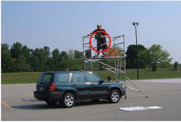
Fig. 1 Vehicle measurement setup (red circle indicates the location of the instruments). (Color online only.)
