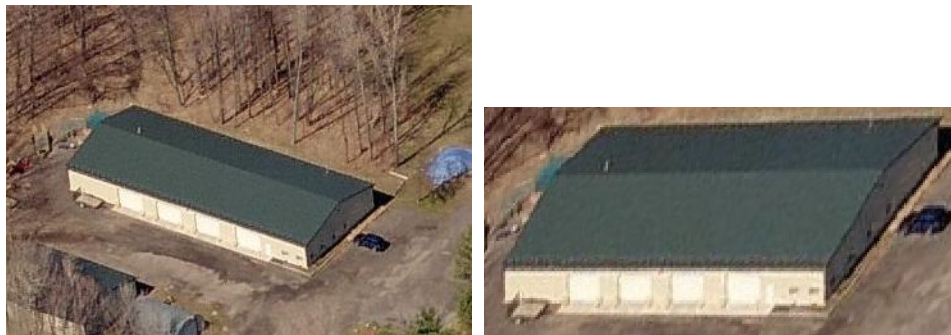
Fig. 8. Oblique image of building, and texture map image for the facet representing the building side Image obtained via [42].
