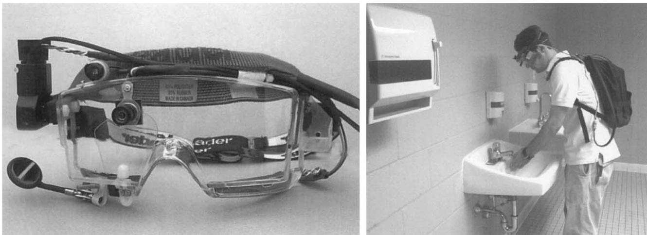
Fig. 1. Left: Headgear contains cameras to image the subject's eye and the scene from the subject's perspective. A semiconductor laser mounted above the eye projects a two-dimensional calibration pattern that remains stable with respect to the subject's head and the scene camera. Right: The controller, display unit, and recording systems are contained in a backpack worn by the subject.
