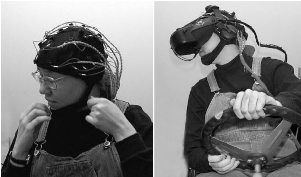
Figure 7 Subject driving with EEG electrode cap
