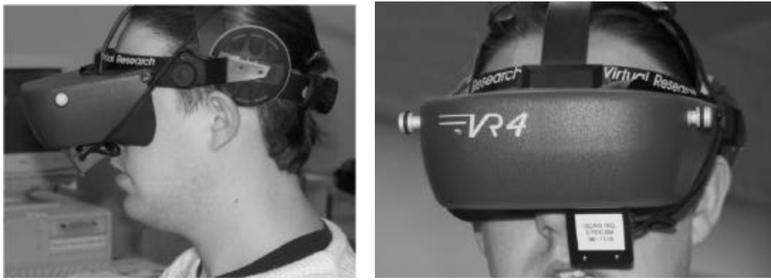
Figure 5 VR4 HMD with integrated ISCAN eyetracker
