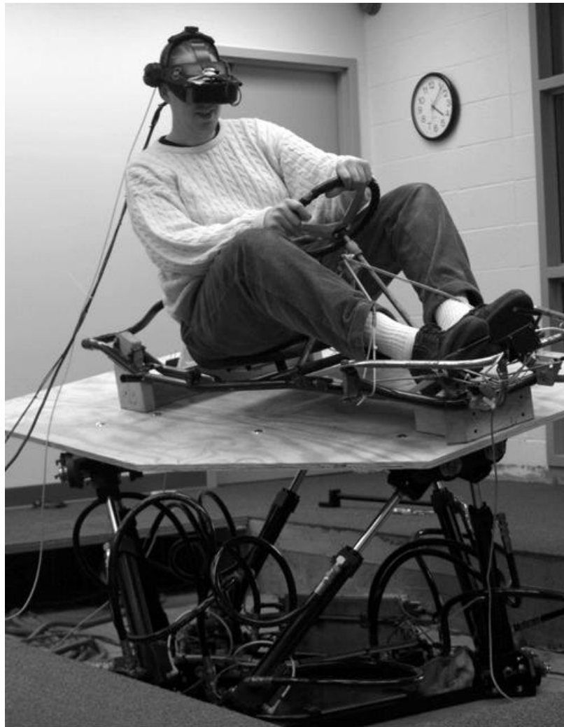
Figure 2 Driving simulator on 6DOF motion platform
