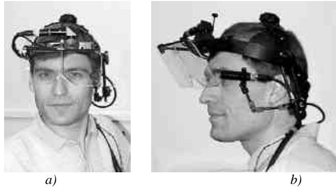
Figure 1 ASL eyetracker headgear. The module above the headband in a ) contains the IR illuminator and eye camera. The visor and scene camera are visible in b ).
