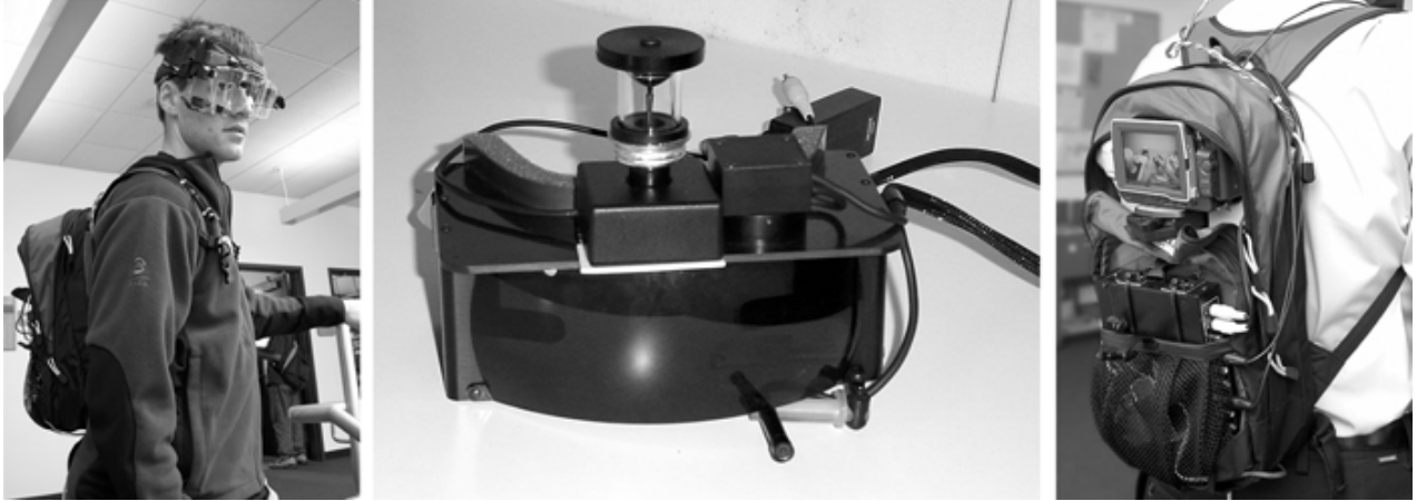
Figure 2: The wearable eye tracker: headgear and backpack, headgear with omnidirectional vision sensor, and detail of backpack.
