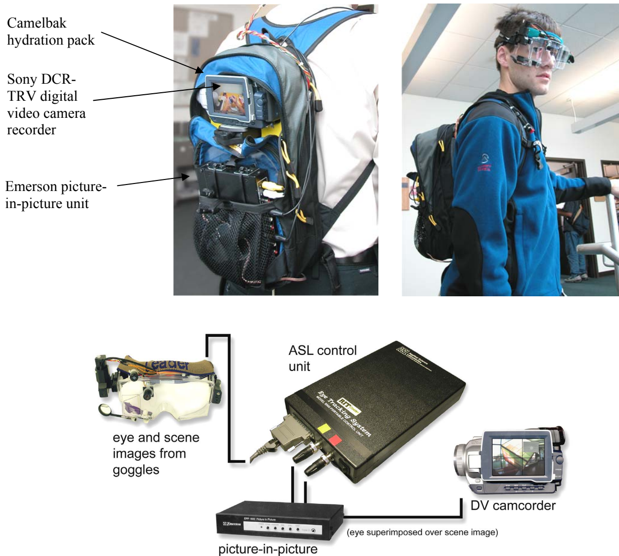
Figure 9 – Top images show a person wearing the RIT portable eye tracking system. Bottom image shows a diagram of the components carried in the backpack.
