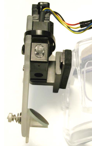
Figure 6b – Folding mirror with controlled image alignment.
