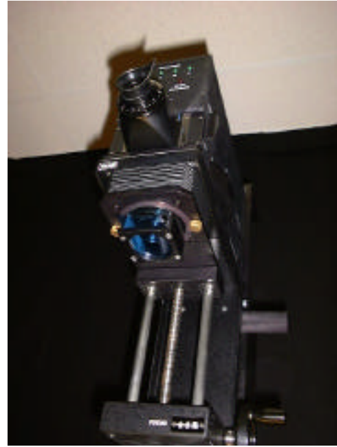
Figure 12b. IBM digital camera head with light blue absorption filter.
