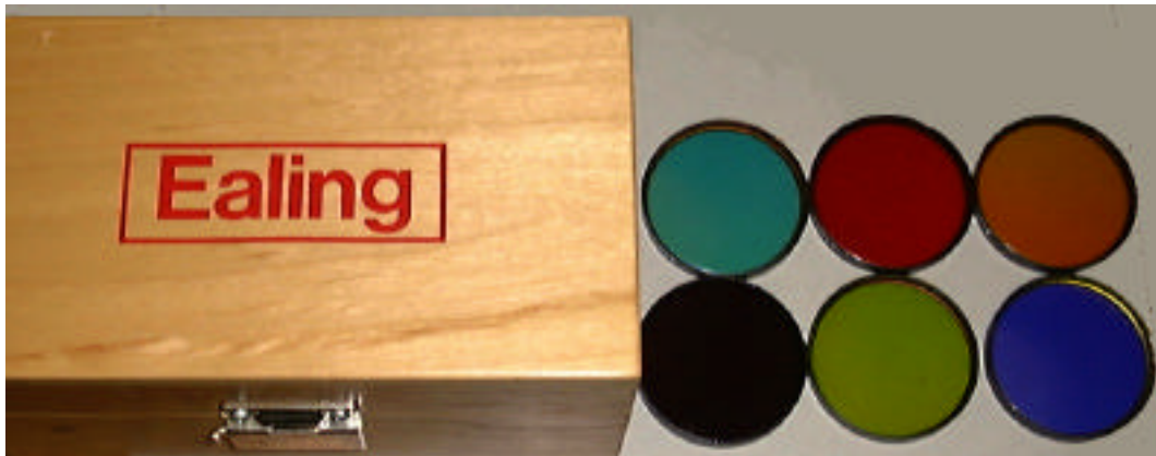
Figure 10. Ealing interference filters used for the narrow-band multi-spectral acquisition.
