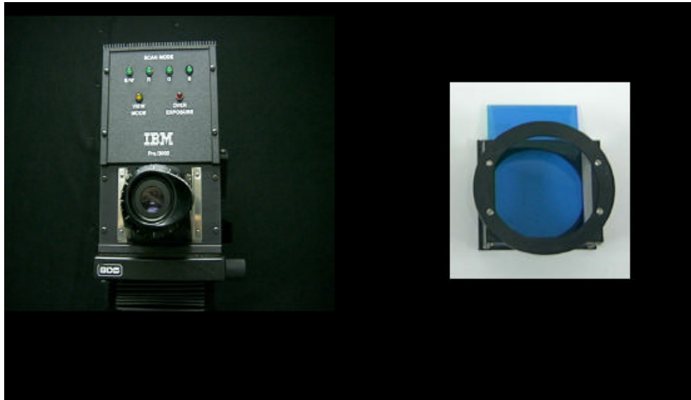
Figure 1. IBM PRO\3000 Digital Camera System head and Kodak Wratten absorption filter with the filter holder.
