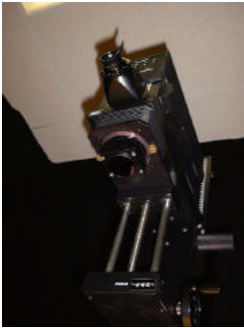
Figure 12a. IBM digital camera head with red interference filter.
