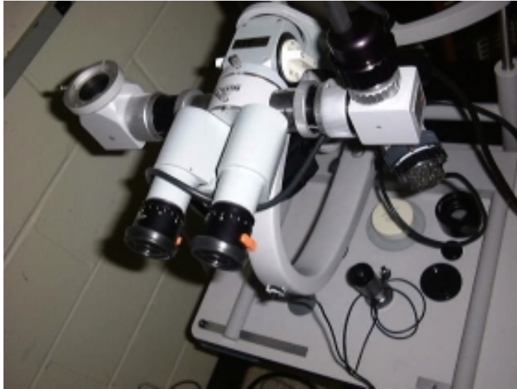
Figure 6. Carl Zeiss Inc. ZVS 1470 slit lamp ophthalmic microscope. Back view showing the multiple-use attachments (for imaging/measurement)
