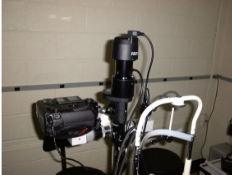
Figure 9. Topcon SL-7E slit lamp ophthalmic microscope with an attached Kodak DCS 620 camera.
