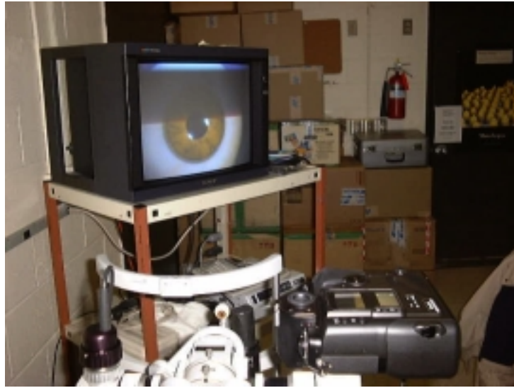
Figure 5. Video signal from the slit lamp displayed on a monitor
