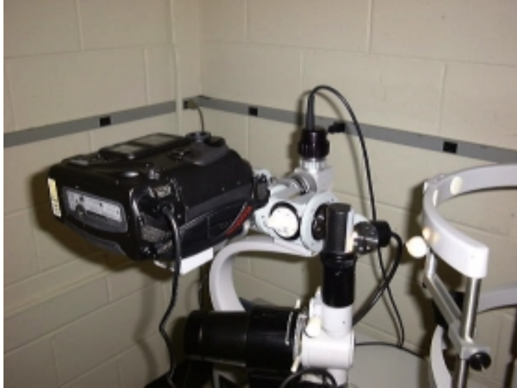
Figure 8. Carl Zeiss Inc. ZVS 1470 slit lamp ophthalmic microscope with an attached Kodak DCS 620 camera.
