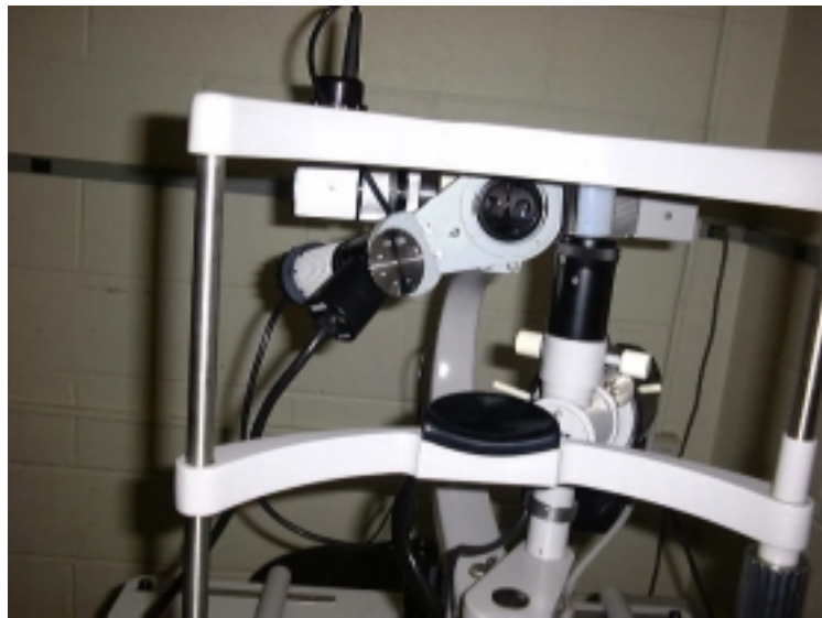
Figure 7. Carl Zeiss Inc. ZVS 1470 slit lamp ophthalmic microscope. Front view showing chin rest and the slit lamp illumination.
