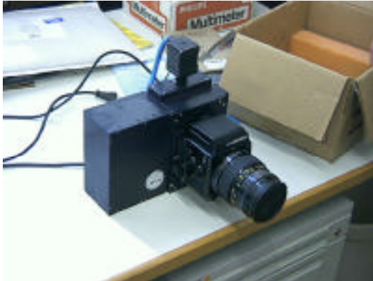
Figure 16. MARC project camera (the digital camera attached to a Bronica camera body) of the Pinakothek, München
