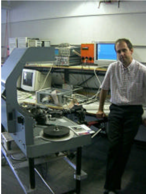
Figure 12. Armin Wittmann and the movie film scanner of the Electronics Laboratory, ETH Zürich
