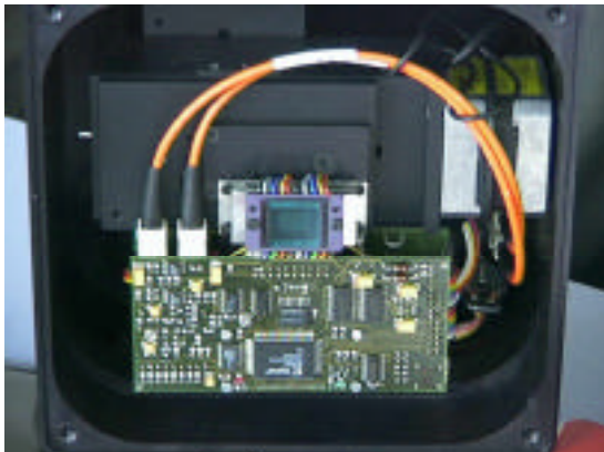
Figure 18. Details of MARC 2 project camera showing electronic board, CCD and cables.
