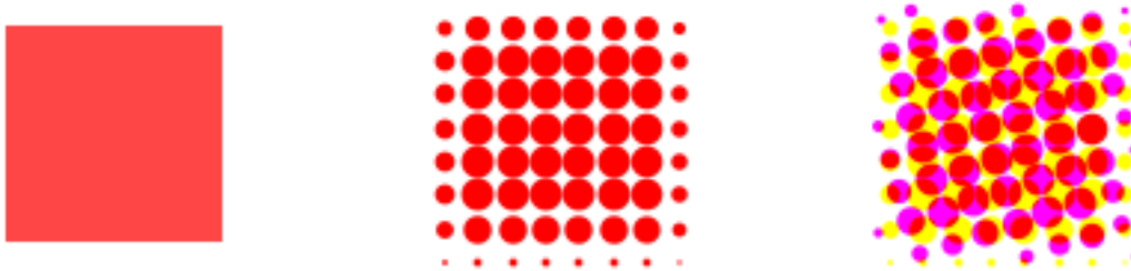
Fig. 3. Halftone representation of continuous-tone color (left) using non-rotated (middle) and conventional rotated (right) screening. (Photoshop stylize plug in used to generate images.)
