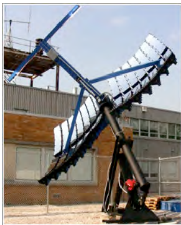
Solar Concentrator System Green Field Solar, Cleveland, OH 5kW, Roof Top (800-1000X)
