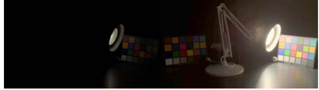
Figure 2. Linear (left) and local-adaptation (right) renderings of the HDR Luxo Double Checker image.
