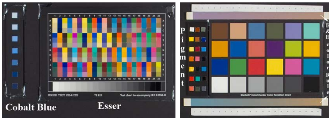
Figure 7. A target consisting Cobalt Blue and Esser (left) and a target consisting Pigment charts, Macbeth ColorChecker, D&H Color Rule.
