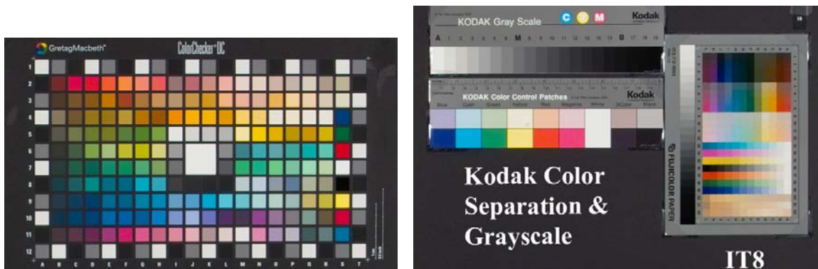
Figure 8. ColorChecker DC (left) and Kodak Color Separation & Grayscale and IT8 (right).
