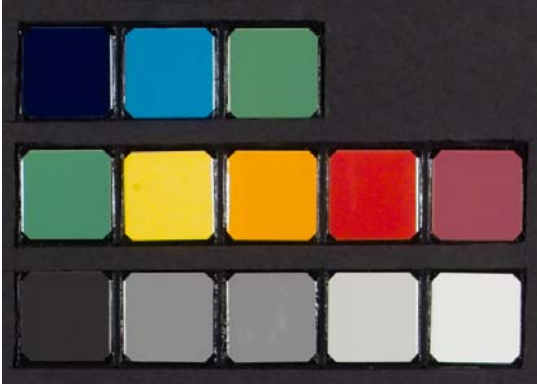
Figure 9. BCRA (British Ceramic Research Association) target.
