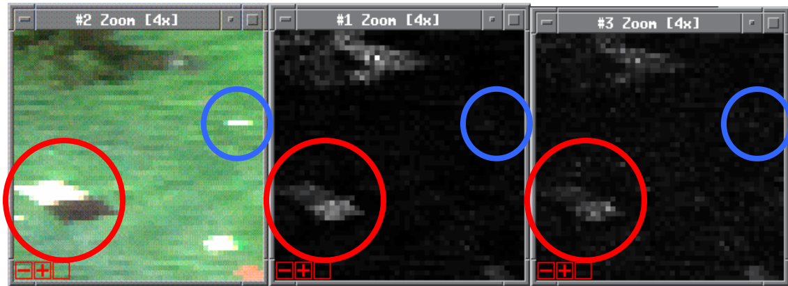
Figure 15: (a) Original true-color image zoomed in on the clean targets (circled in red) and the contaminated targets (circled in blue). (b) & (c) Probability maps zoomed in on the clean targets and the contaminated targets (also circled in red and blue respectively). The first was created using the default parameter values (8 MaxD vectors and 3 FSR vectors) and the second was created using the parameters found to be ideal for the AVIRIS data (30 MaxD vectors and 15 FSR vectors).
