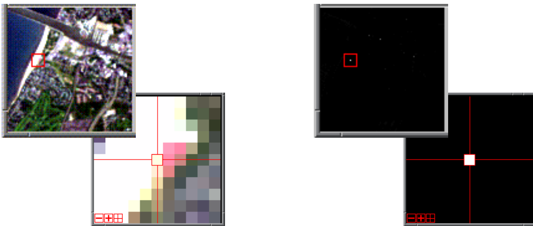
Figure 10: (a) True color image zoomed into what was considered the target pixel. (b) The probability map and target pixel resulting with the use of 25 FSR vectors.
