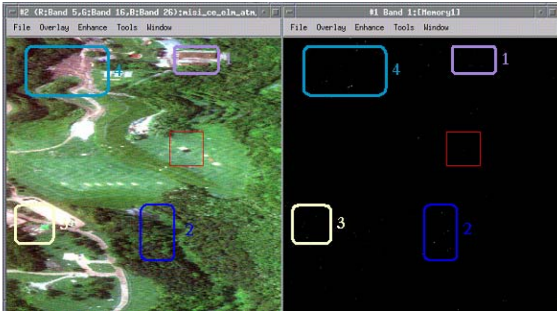
Figure 12: (a) The true-color MISI image used for testing the effectiveness of MaxD and the Invariant Algorithm on concealed and contaminated targets. (b) Resulting probability map with circled areas of high false alarms.
