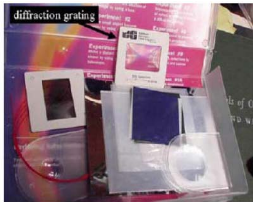
Figure 2: Diffraction Grating in OSA Optics Discovery Kit
