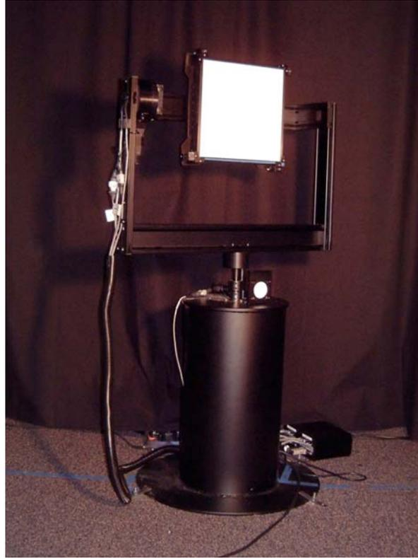
Figure 8. Three-Axis Sample Positioner as installed in the MCSL Spectral Imaging System. A 12x12" Fluorilon white reference has been mounted on the positioner; the round white pressed Halon reference used for illumination monitoring is at the top of the base and the two Velmex motor controllers are visible on the floor.
